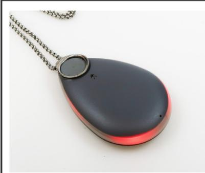
The light-ring around Chiptech GO will flash red to let you know an alert is being sent to the Alarm Receiving Centre (ARC). A voice message will play, "Help alert in progress."
